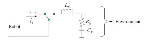
The switch can be controlled by the position:  $\int_0^t i_1(t) dt$
