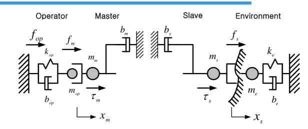
The dynamics of the master arm and slave arm is given by the following equations
