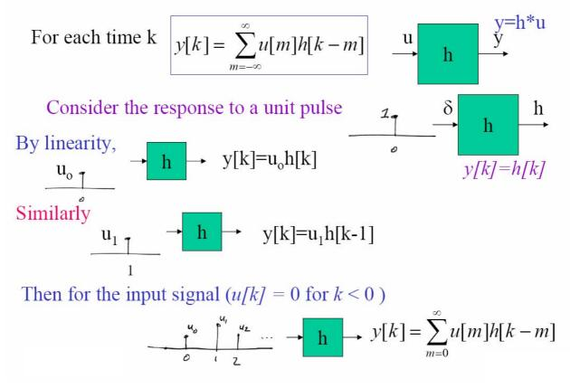
The input-output characteristics of an LTI system are completely described by the impulse response *h*[*n*].
