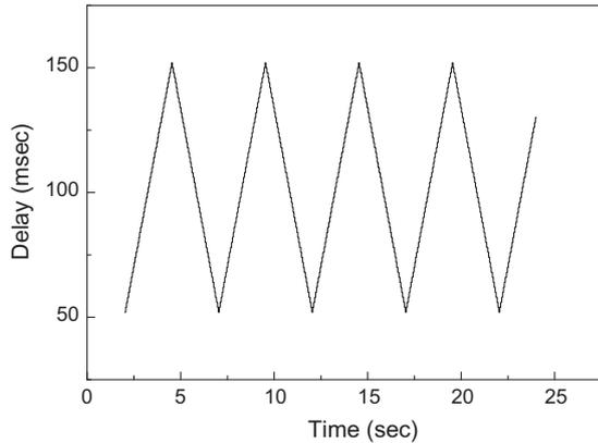
Fig. 12. Amount of time-varying delay during the experiment. An average round trip delay was 100 ms and varied between 150 ms and 50 ms.
