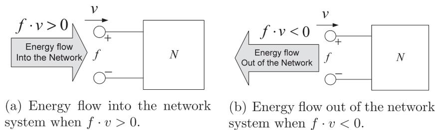
Fig. 5. Based on the sign of the power at a port, it is possible to differentiate whether energy is flowing into the network system or flowing out of the network system.
