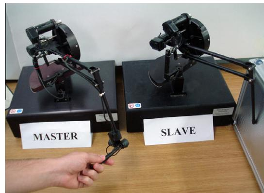
Fig. 11. Dual PHANTOM for the teleoperation with time-delay.
