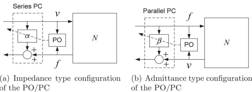
Fig. 2. Impedance and admittance type configuration of the Passivity Controller for a one-port network system.
