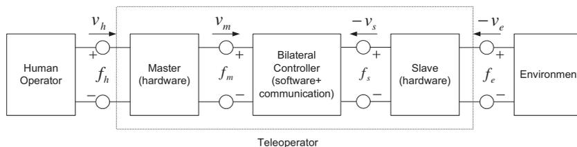
Fig. 3. Block diagram of a complete teleoperation system.
