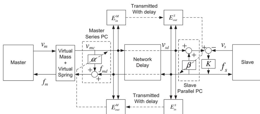
Fig. 10. A time-delayed teleoperator with the proposed two-port TDPA and the virtual mass with spring.
