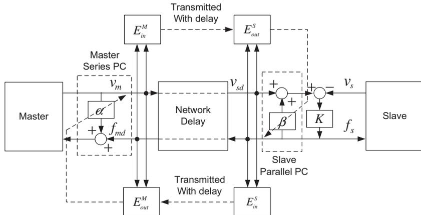
Fig. 8. A time-delayed teleoperator with the proposed two-port PO/PC.
