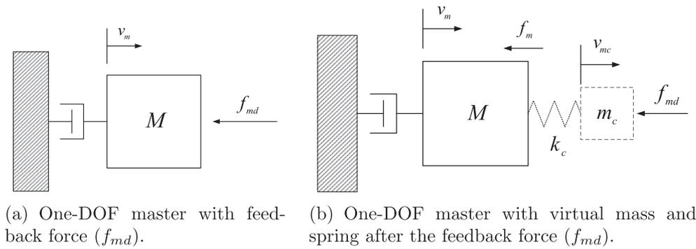
Fig. 9. Comparison of one-DOF master with and without virtual mass and spring.
