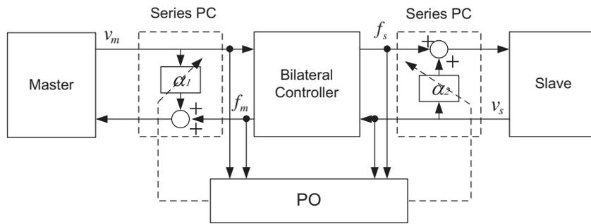
Fig. 4. Block diagram of a teleoperator with PC. Two series PCs are attached at each port of the bilateral controller.
