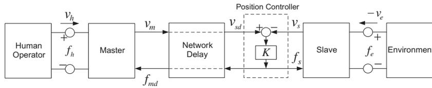
Fig. 7. A time-delayed teleoperation system with position-force bilateral control architecture.
