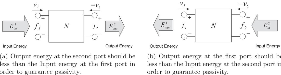
Fig. 6. In two-port network systems, the main source of the output energy at one-port is the input energy at the other port, and the output energy should be less than the input energy.
