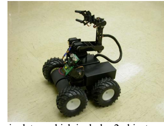
Fig. 3. Mobile manipulator, which includes 2 objects: mobile platform and robotic arm. They are easy to be controlled independently by the use of switching of control signals.
