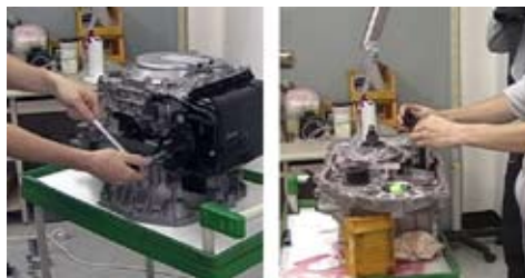
Fig. 3 Conventional disassembling process
