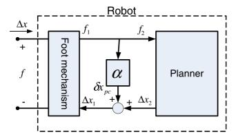
Fig. 4. One-port network with PO/PC.
