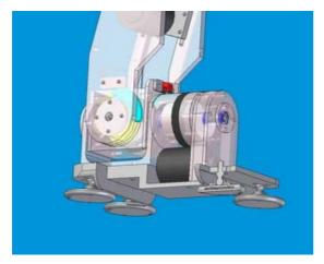
(a) Foot structure with four FSRs.
