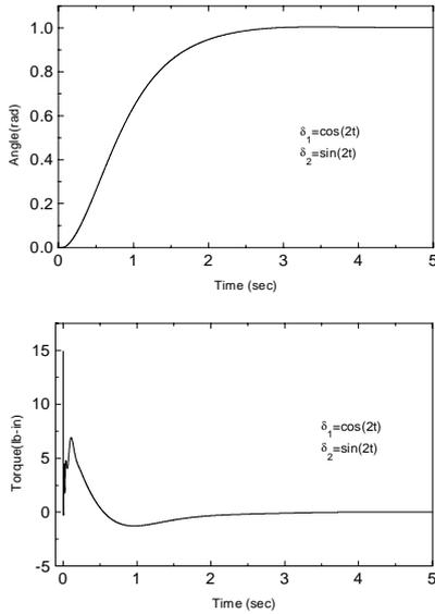
Fig. 2. Robust Performance of time-varying uncertainty (Step response)
