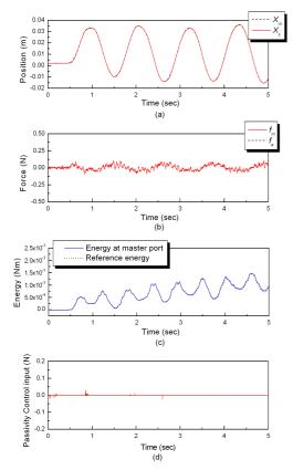
Fig. 7. Experimental result: unconstrained motion of master/slave teleoperation system with the proposed reference energy following scheme with the PC.
