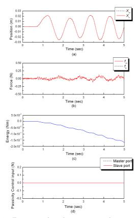
Fig. 4. Experimental result: unconstrained motion of the master and slave teleoperation system without the PC. The PO value was kept falling down to more negative value even though the response was stable.
