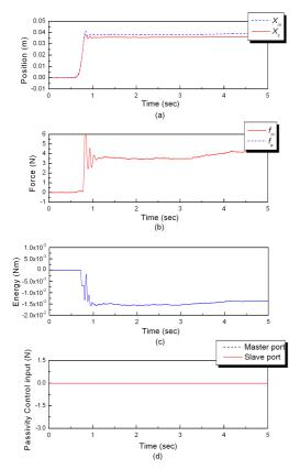
Fig. 5. Experimental result: Operator maneuvered the master to make the slave contact with a soft sponge without the PC. The PO value crossed to negative values even though the contact response was stable.
