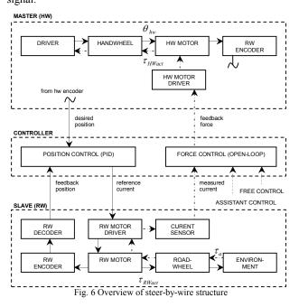
When the RW DC motor actuates the roadwheels accordingly, a proportional current signal inside the motor driver of occurs at the same time. Fortunately, the value of the current signal depends on the load applied on motor shaft because of the current-torque relationship of DC motors.
