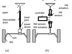
Fig. 1 Conversion from conventional steering system to SBW
