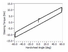
Fig. 9. HW position vs. Force feedback with tire-to-ground contact The final force feedback is achieved after introduction of assistant torque based on HW angle and vehicle velocity, Fig. 10.
