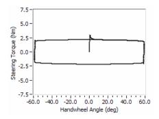
Fig. 8. HW position vs. Force feedback without tire-to-ground contact
