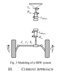
In this section, we focus on the force feedback implementation for the SBW systems. Normally, the force feedback known as driving feelings is from the RW part. This includes moment of inertia and damping; align moment, joints' friction. The feedback force is also affected by tire properties, road condition, vehicle velocity, and so on.
