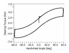
Fig. 10. HW position vs. Force feedback with assistant torque
