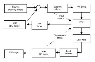
Fig. 4 Control scheme of the torque map method Angle effect term:
