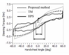
Fig. 11. Comparison of proposed method and others HPS: hydraulic power steering, TM: torque-map method
