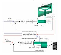
Fig. 5 Position-force control scheme
