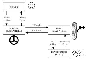
Fig. 2 SBW is considered as a two-port network
