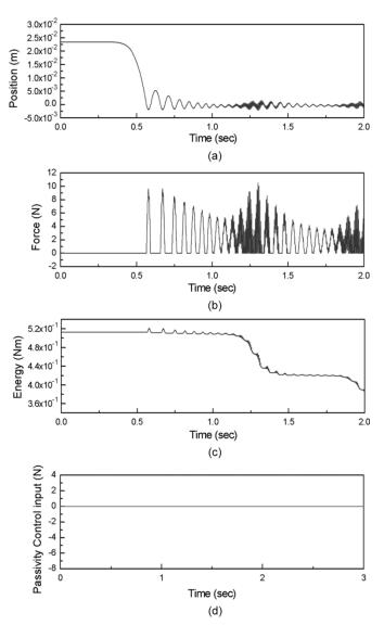
Fig. 11. Experimental results. Contact response with the PO/PC without resetting and reference energy.
