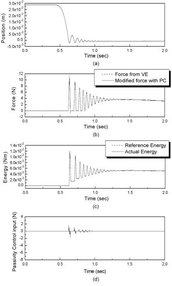
Fig. 10. Experimental results. Contact response with the PO/PC with reference energy without model for high stiffness VE (K = 5000 N/m).
