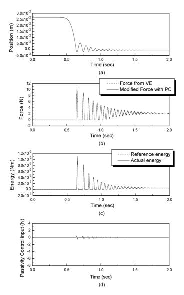
Fig. 9. Experimental results. Contact response with the PO/PC with reference energy based on model for high stiffness VE (K = 5000 N/m).
