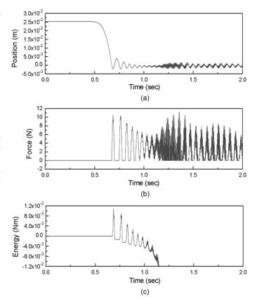
Fig. 2. Experimental results. Contact response without the PO/PC for high stiffness VE (K = 5000 N/m).
