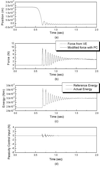
Fig. 12. Experimental results. Contact response with the PO/PC without resetting and with reference energy.
