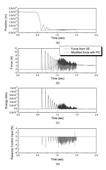
Fig. 3. Experimental results. Contact response with the PO/PC for high stiffness VE (K = 5000 N/m). Although contact is now stable, transient behavior is poor.
