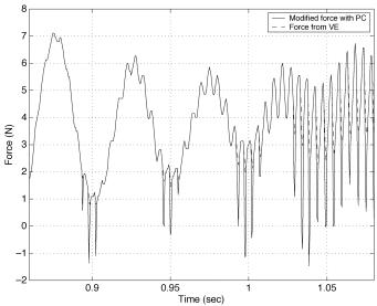
Fig. 6. Experimental results. Impulsive PC control action makes the internal mode vibrate.
