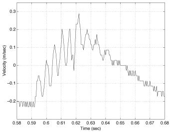
Fig. 4. Experimental results. Velocity behavior during the contact, 200 Hz internal mode.
