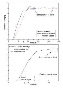
Fig. 5. Experimental results for mobile robot positioning when only textual feedback is provided to human-operator.
