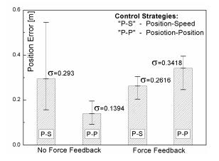
Fig. 9. Position error diagram for different control strategies with and without force feedback.
