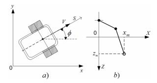
Fig. 1. Configurations of a two-wheeled mobile robot (a) and a master device (b).
