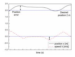
Fig. 7. Positioning error in teleoperation.
