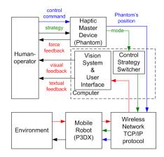
Fig. 2. Architecture of the experimental setup.
