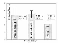
Fig. 6. Navigation time diagram for different control strategies.
