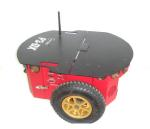
Fig. 4. Mobile robot Pioneer 3-DX from MobileRobots, Inc.
